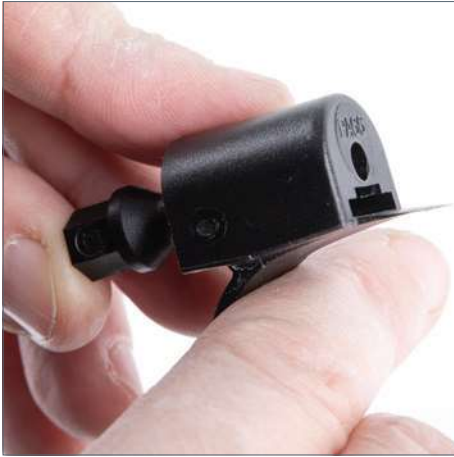
Insert Screw into Housing
